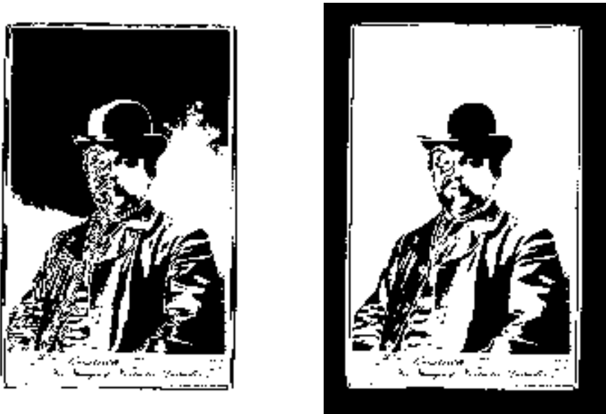
Figure 7.10: The binary (left column) and Gray code (right column) of bit plane 5 of the image in Fig. 7.1 .
