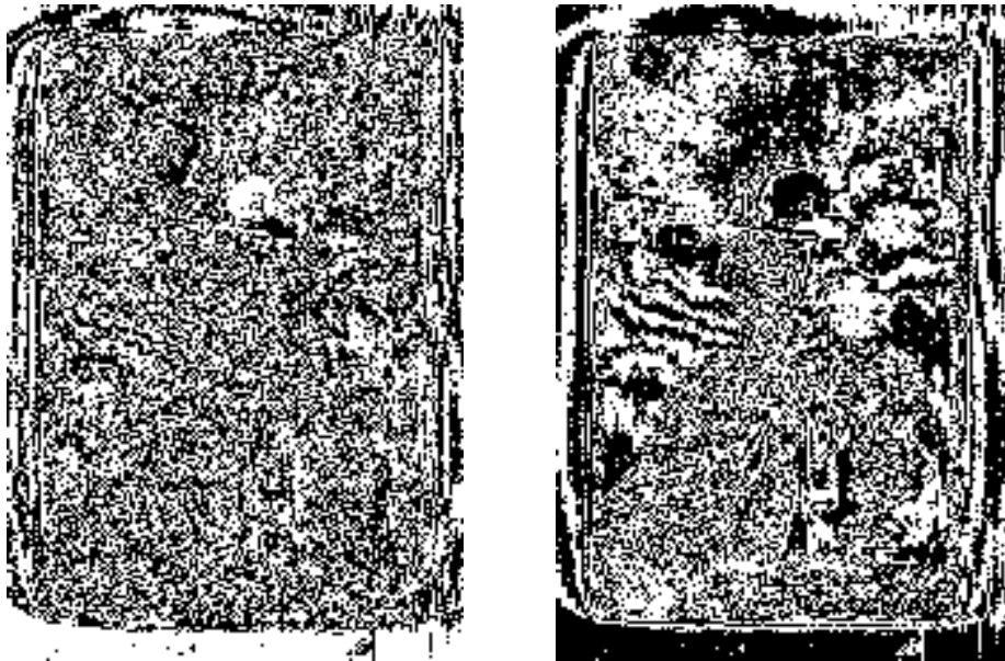
Figure 7.6: The binary (left column) and Gray code (right column) of bit plane 1 of the image in Fig. 7.1 .
