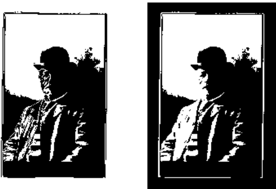
Figure 7.11: The binary (left column) and Gray code (right column) of bit plane 6 of the image in Fig. 7.1 .
