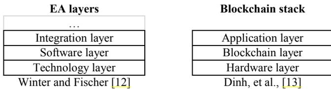
Fig. 1. Enterprise Architecture layers and the blockchain stack.
