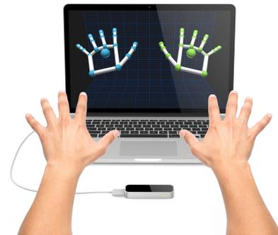
Figure 3.2: Visualization of hands on a PC using the Leap Motion controller.
