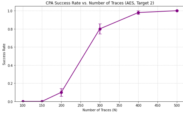
Figure 7: Success rate (over 50 iterations) for varying numbers of power traces when attacking AES on Target 2
