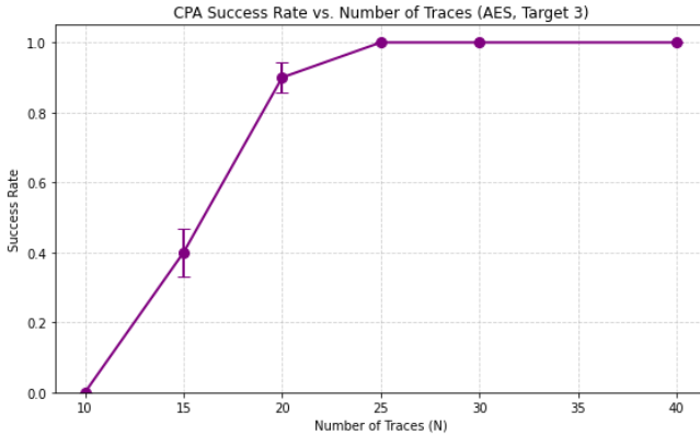
Figure 9: Success rate (over 50 iterations) for varying numbers of power traces when attacking AES on Target 3
