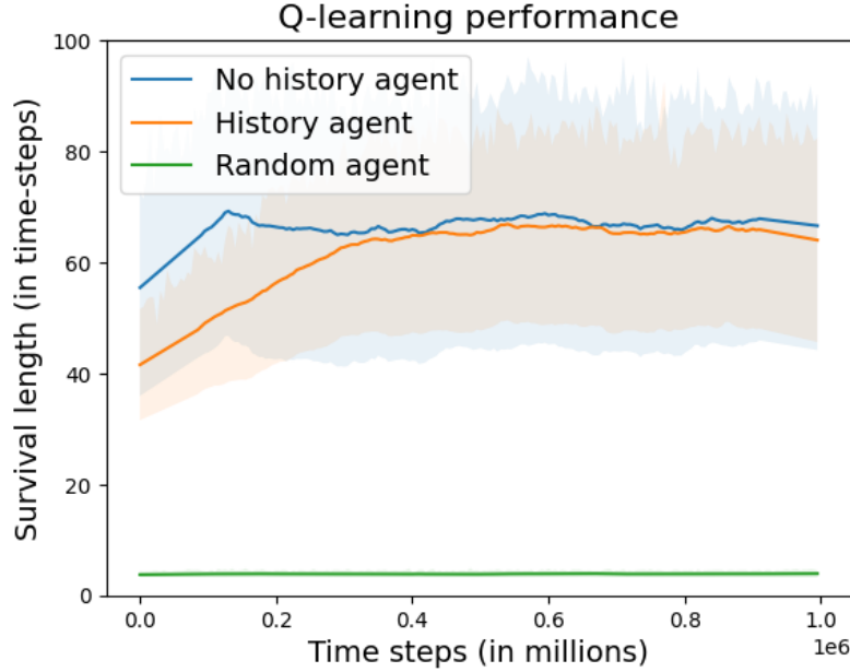
Figure 2: Q-learning algorithm performance on a 3x3 lattice with a bit-flip error rate of 0.01 with 0.01 drift, comparing a Q-learning agent that uses only the current observation with a Q-learning agent that uses both the current and previous observation as a state representation. We see that the performance of both agents is very similar towards the final evaluations, but the history agent is slightly outperformed.
