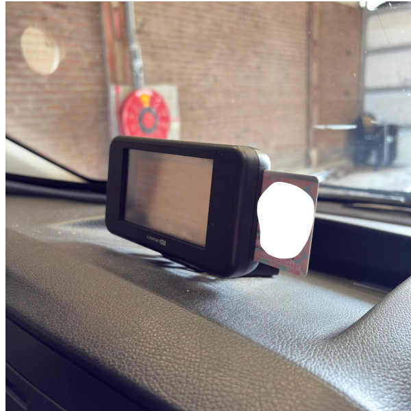
Figure 1: Driver inserts the driver card into the BCT to log in at the start of a shift.
