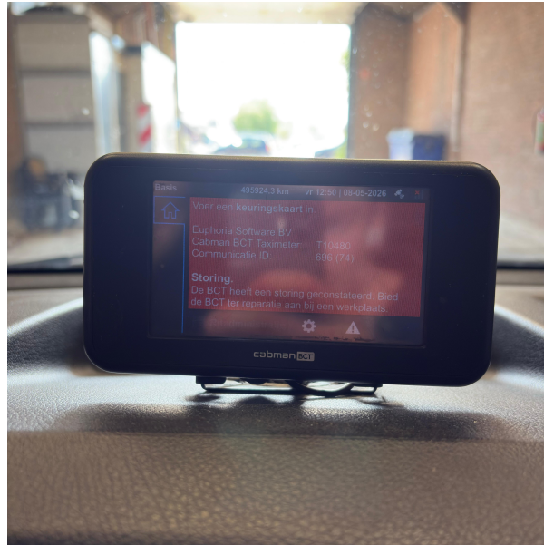
Figure 2: The BCT displays a malfunction notice during a shift.
