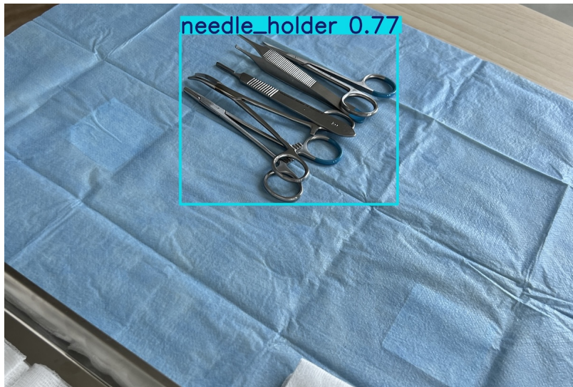
Figure 14. Failure case for overlapping multiple tools detection. Multiple instruments are grouped into a single detection and jointly classified as a needle holder, rather than being separated into distinct instances.
