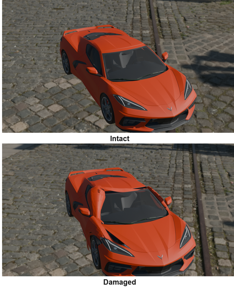
Figure 5: A representative vehicle from the generated dataset, rendered intact (top) and with procedural displacement damage (bottom) from the same viewpoint, under domain-randomized lighting and backgrounds. The damage appears as a localised deformation of the front-left panel, distinct from the smooth intact surface.
