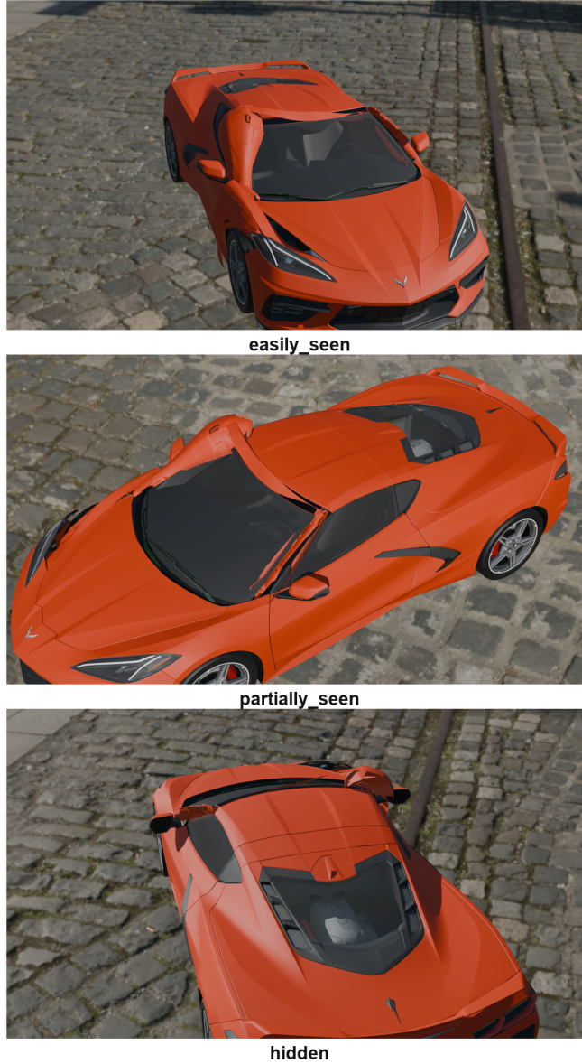
Figure 6: The same front-zone damage on one vehicle at the three observability levels assigned by the generator: easily_seen (top, camera facing the damage), partially_seen (middle, camera to the side), and hidden (bottom, camera opposite). The deformation is prominent from the facing viewpoint, partial from the side, and absent from the opposite one.
