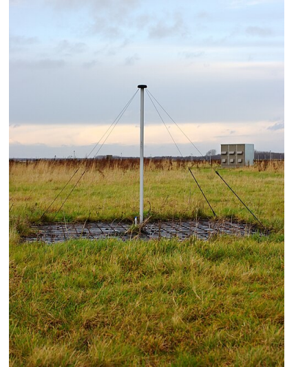
Figure 3: A low-band antenna (LBA) of the Low-Frequency Array (LOFAR). The LOFAR cabin containing the electronics is visible in the background right. 2
