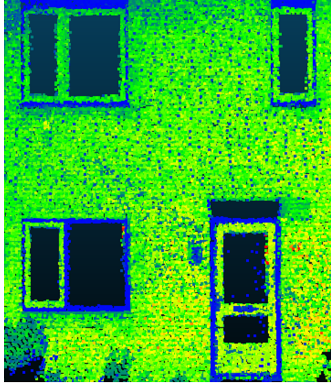
Figure 12: Windows, doors, and their respective frames are clearly separated based on intensity information, showing distinct regional boundaries.
