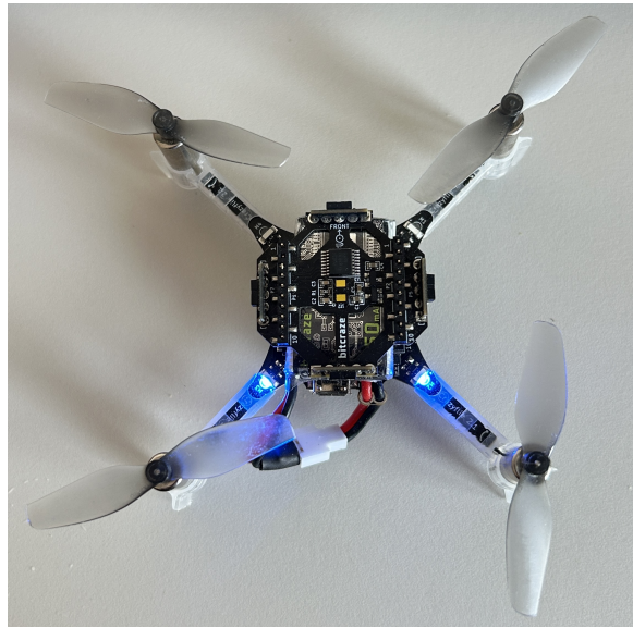
Figure 7: The Crazyflie 2.1+ is equipped with a Flow Deck and Multi-Ranger Deck for onboard sensing.
