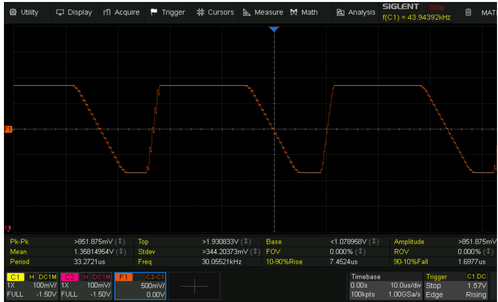
Figure 12: Resulting waveform of periodic heating from 30 kHz pulses with constant -0.1 V cooling
