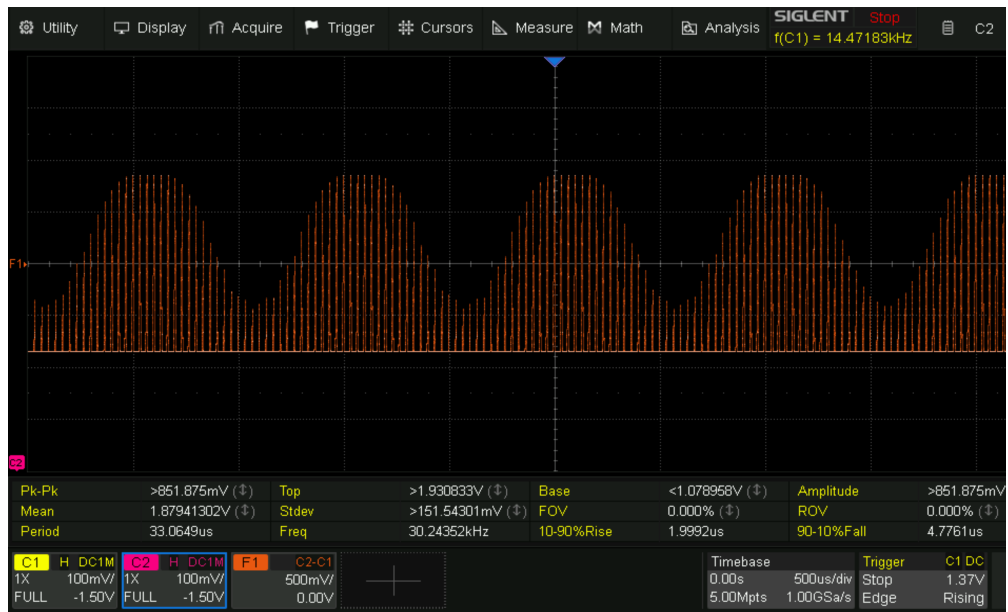
Figure 14: Resulting waveform of periodic heating from 30 kHz pulses with sine wave cooling
