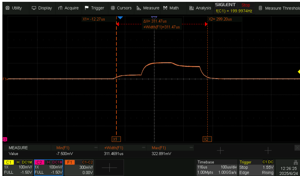
Figure 10: Resulting waveform of the heat equation with decreased negative feedback, a low integration constant and two overlapping pulses
