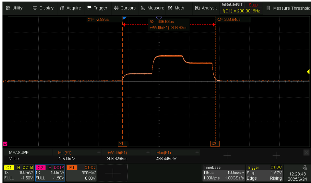
Figure 7: Resulting waveform of the heat equation with two overlapping pulses
