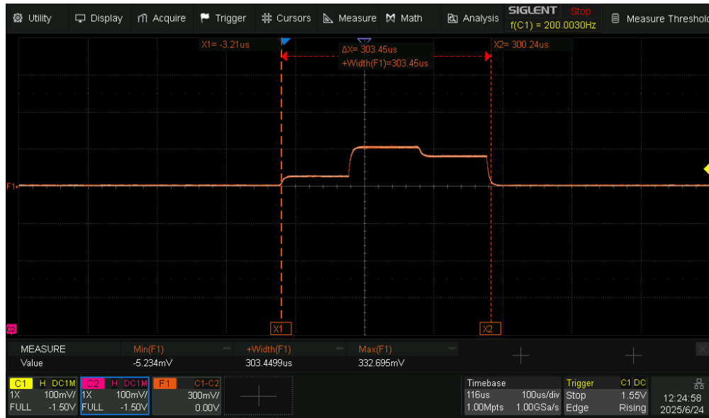
Figure 9: Resulting waveform of the heat equation with increased negative feedback and two overlapping pulses
