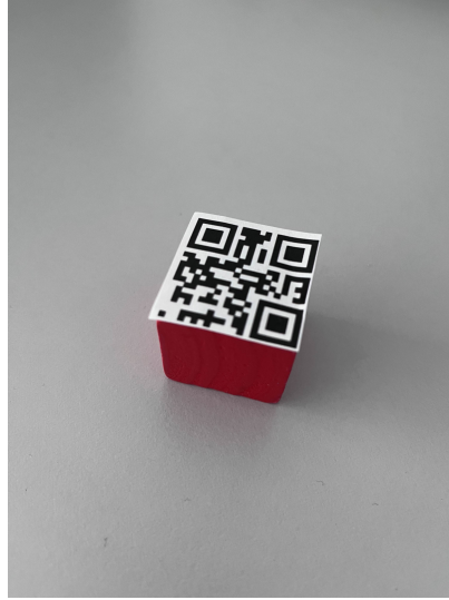
Figure 10: Cube with a QR code stuck on top. The content of the QR code does not impact the use of this method and can be anything. In this case reading the QR code returns the message "I am a cube"
