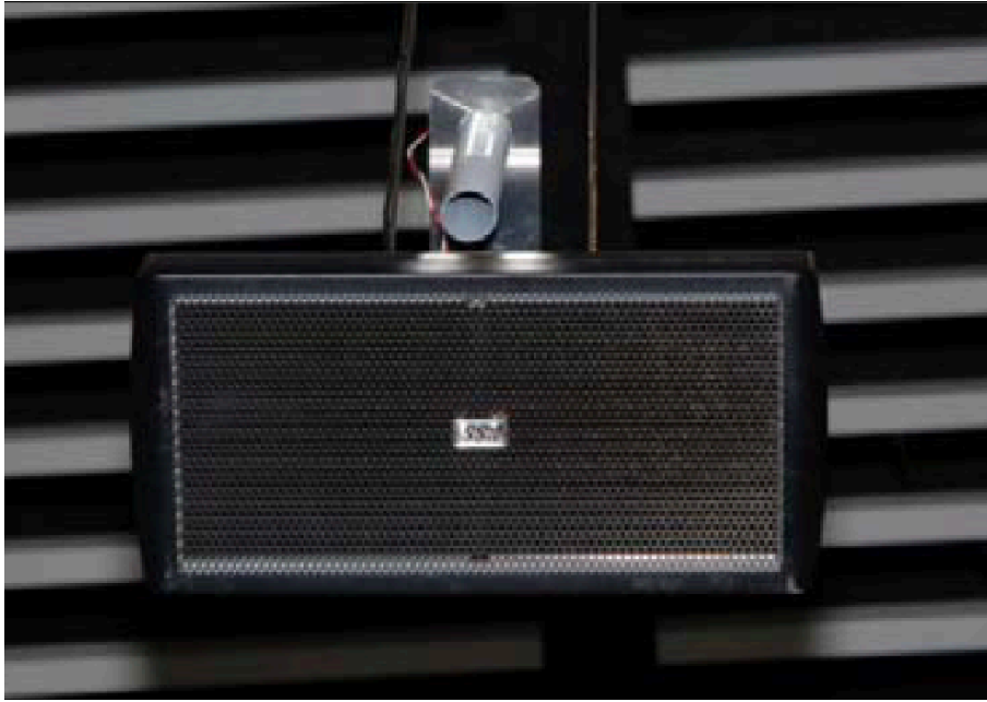
Figure 7: Directional speaker and a PIR sensor. (Kortbek & Grnbk, 2008)
