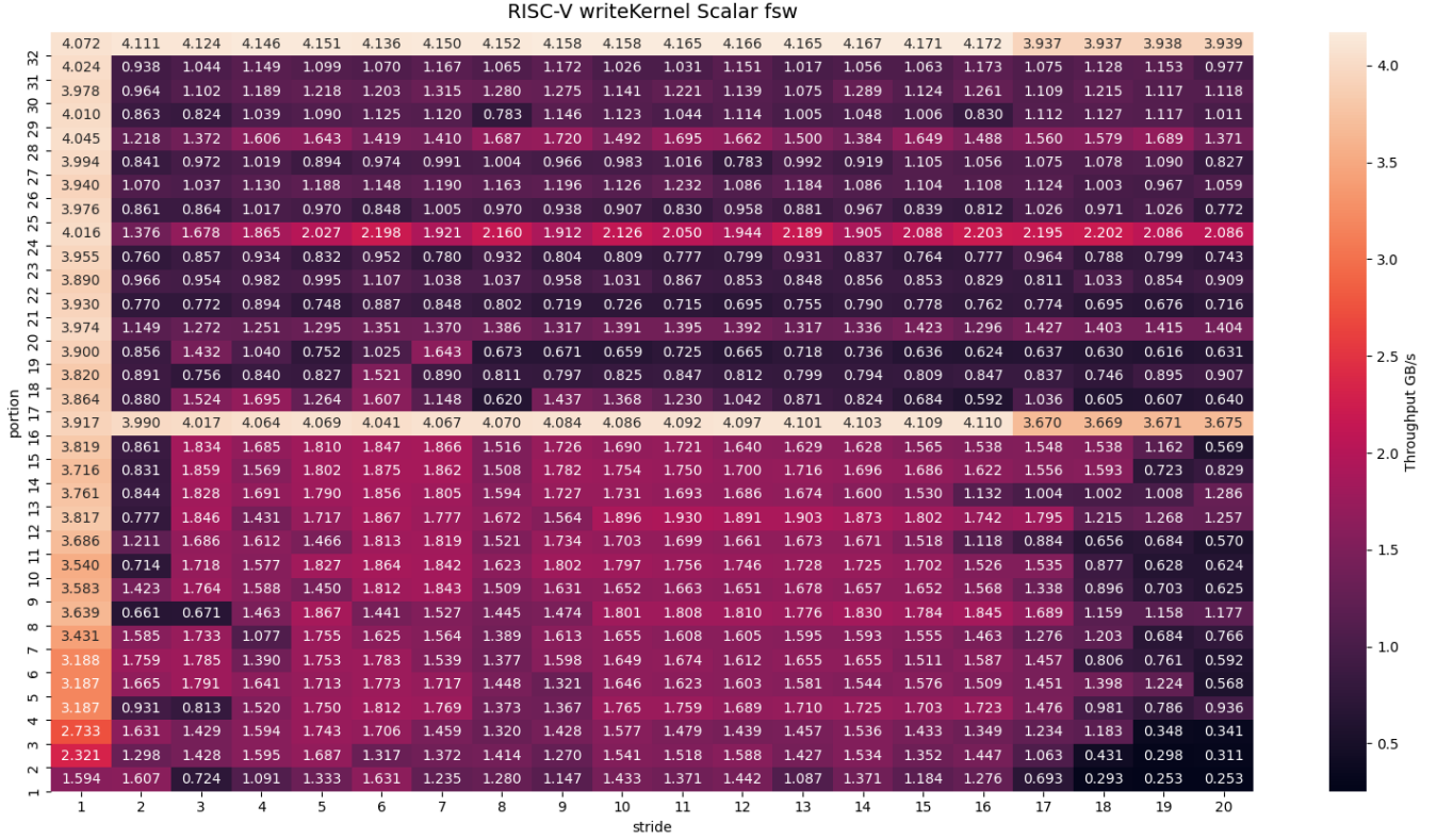
Figure 11: Throughput (GB/s) per striding configuration for writeKernel using scalar registers with single-precision floating points and instruction fsw for the RISC-V SpacemiT K1.
