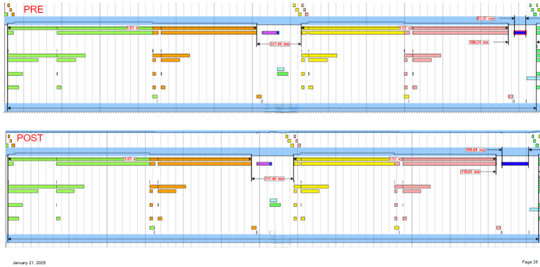
Figure 4: Gantt chart of processes. The bars represent the different processes that happen in Lithography machine while manufacturing a chip.
