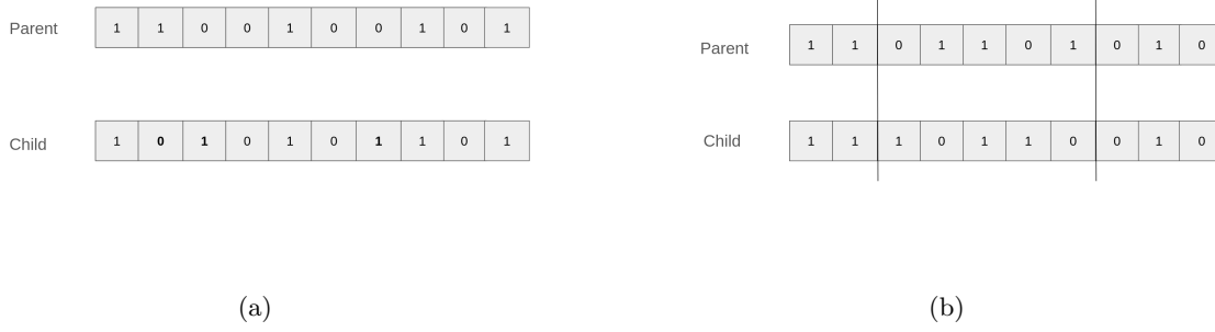
Figure 8: Examples of bit flip(a) and inversion (b) mutation operators.
