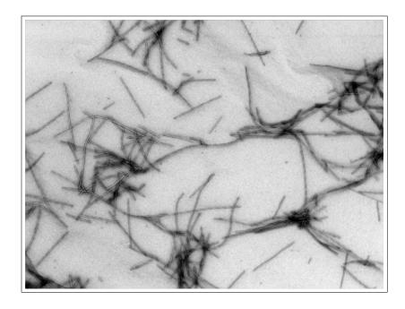
Note. The image illustrates the dense clustering and overlapping of amyloid fibres, which pose challenges for measurements. The dimensions of the image are around  $5.82 \times 4.37$  µm, at a resolution of around 1.766 nm per pixel.
