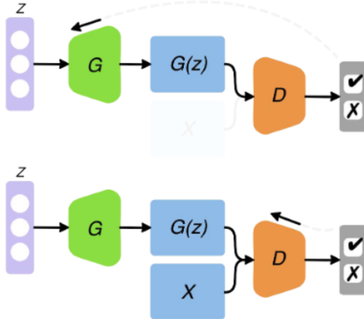
Figure 2: Schematic of the GAN training process[18]. In each training step, the generator G produces fake data from random noise z , and the discriminator D attempts to distinguish this from real data X . Feedback from the discriminator is used to improve the generator. The networks are trained in alternation to push each other to improve.
