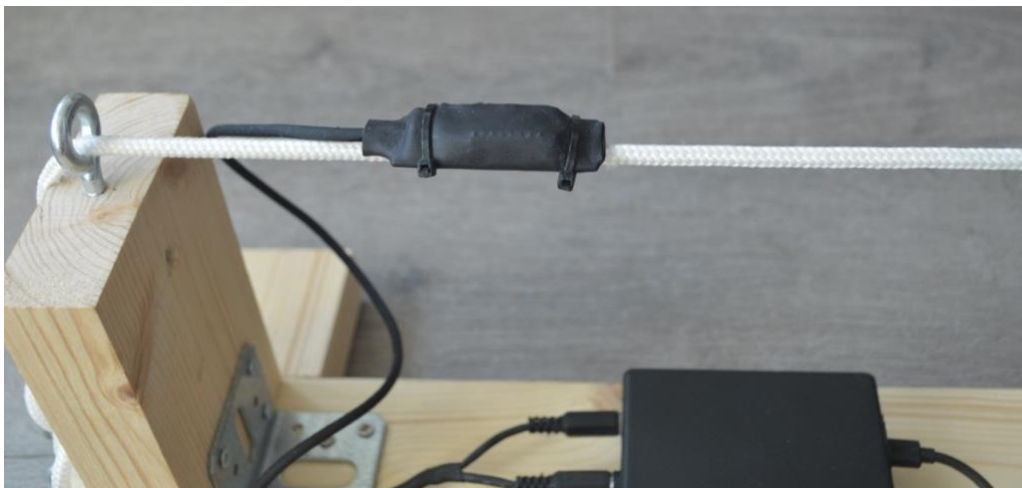
Figure 2: the ROPE - STRING interface, showing below a detail of the motion sensor on one side of the rope.
