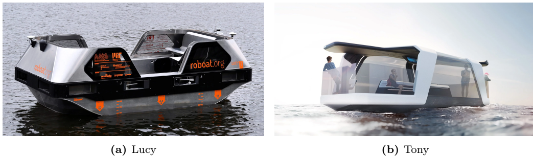
Figure 2: Roboat’s test vessels. a) An image of Lucy which is a small 6-person water-taxi designed for research and demonstration purposes. b) A render of Tony, a larger ferry designed with a maximum capacity of 35 people for supervised autonomous operation on the Seine in Paris.
