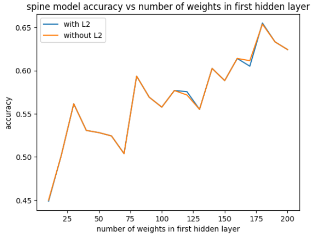
Figure 19: Results when attacking on Spine model with different numbers of parameters (weights) in the first layer.
