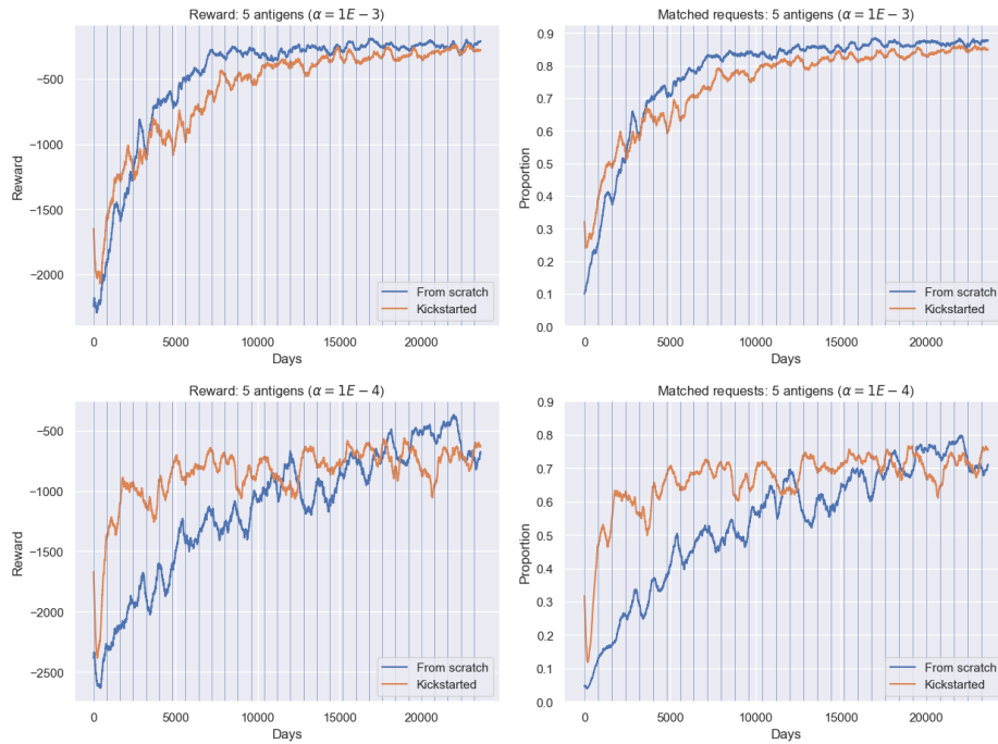
Fig. 10. Daily total training reward (left) and proportion matched requests (right) with ‘kick-starting’ the Q-network in the 5-antigen setting. Learning rates 1E - 3 and 1 * E - 4 were tested. Training was performed for 50 episodes.
