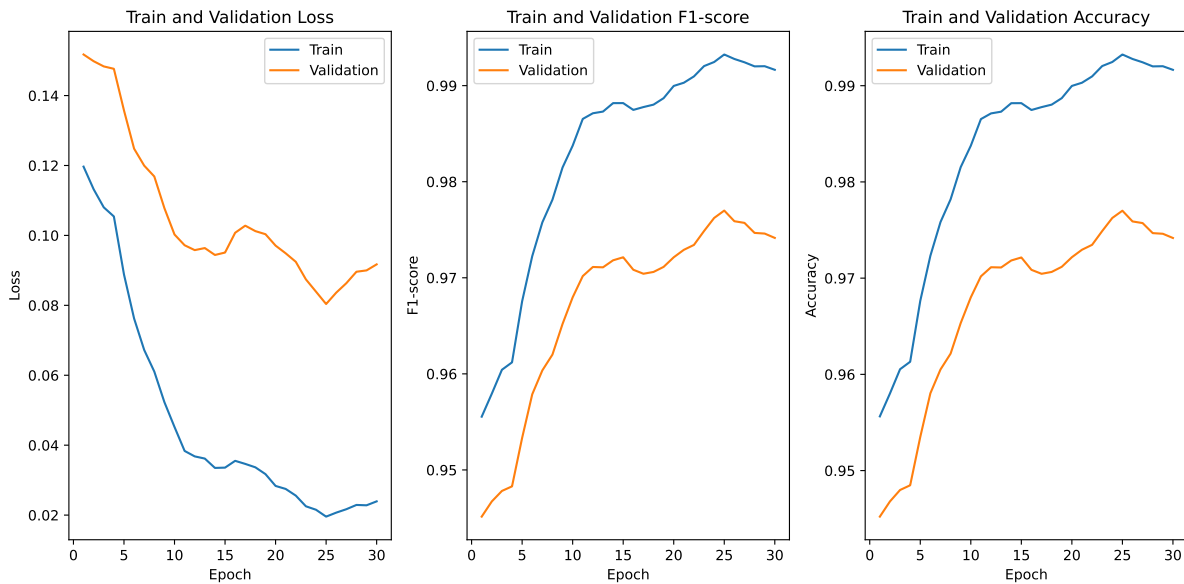
Figure 10: These graphs represent the pre-trained ResNet3D model with 4 optimal frames. On the test set this model achieved a F1-score of 98.0%, accuracy score of 98.0% and a loss of 0.055.
