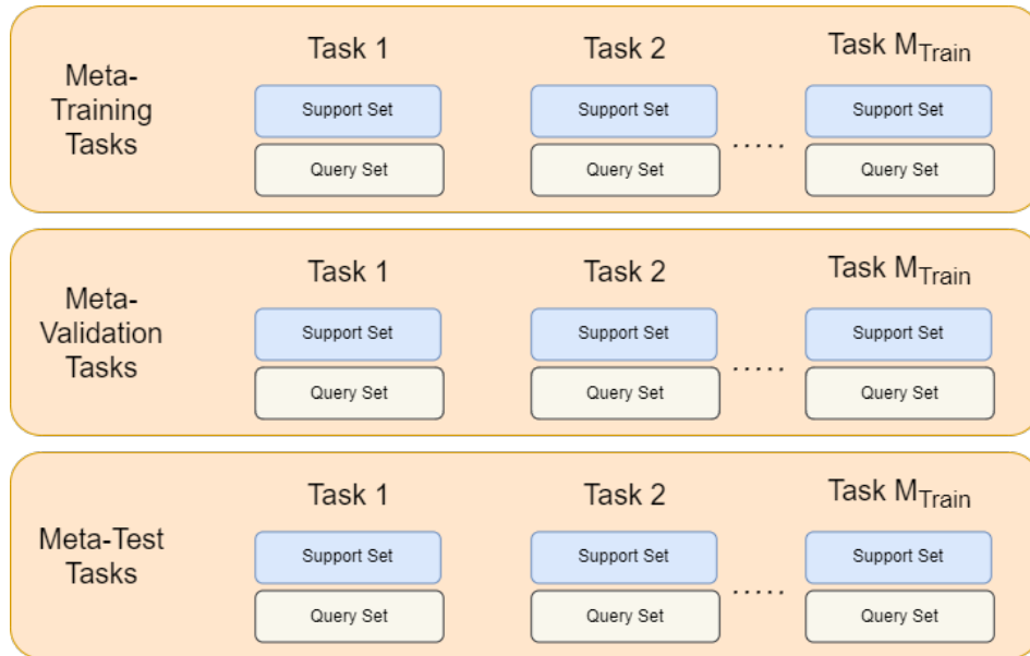
Figure 2: An example of a few-shot learning setup. During meta-training various tasks ( 1, \dots, M , with M referring to the total number of tasks exposed to the model, typically 600) as illustrated in Figure 1 are used to train a model with a disjoint set of tasks sampled from the dataset used for validation. During meta-testing, the test tasks are used for the performance evaluation of the model. Graphic inspired by Ravi and Larochelle [55].
