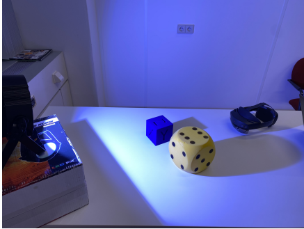
Figure 14: Setup 2- Varying light angles and intensity as well as object position
