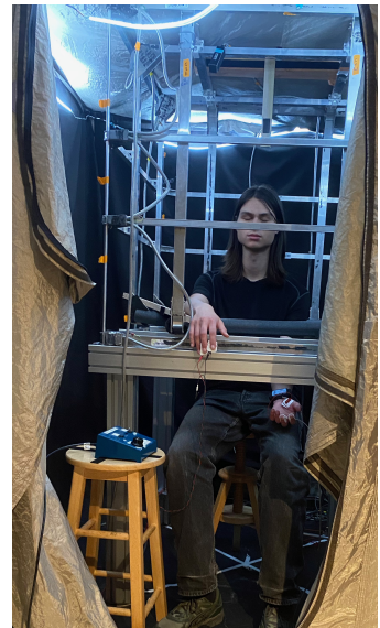
(c) The experimental setup with the subject connected to both the EDA measuring equipment on the non-dominant hand and the shock delivery system on the right hand.
