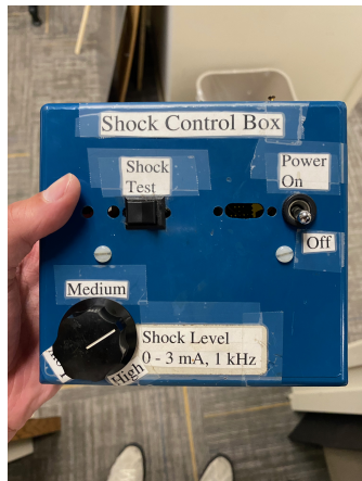
(a) Shock Control Box including a shock level dial (0-3mA) and test trigger.
