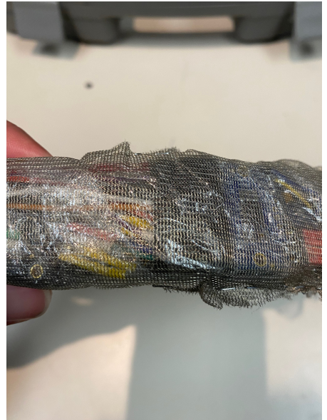
(c) The copper mesh fabric shielding embedded around the MESSy headband
