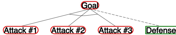
Figure 7: ADT Example with AND refinement and a direct counter child node. Made using the ADT WebApp [5].
