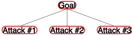
Figure 3: ADT Example with OR refinement and no counter child node. Made using the ADT WebApp [5].
