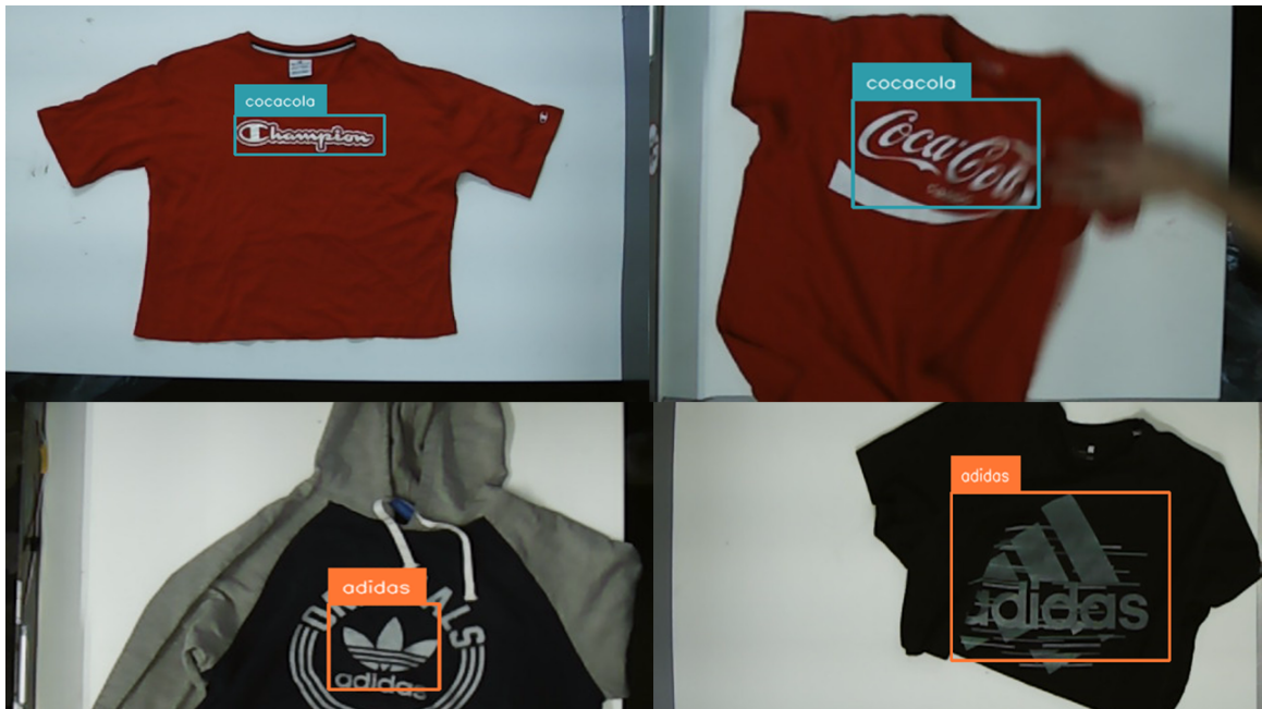
Figure 12: Logo bounding box detections made by the Roboflow model. Here we see three correct predictions and one incorrect prediction. As seen from the top two images, the similarity in colour
