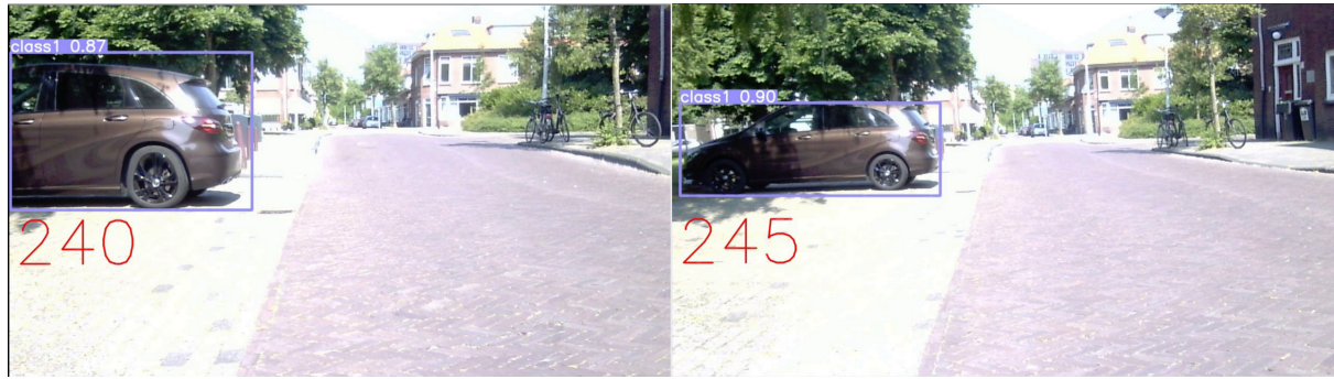
Figure 4: Problematic situation with sideways parked cars
