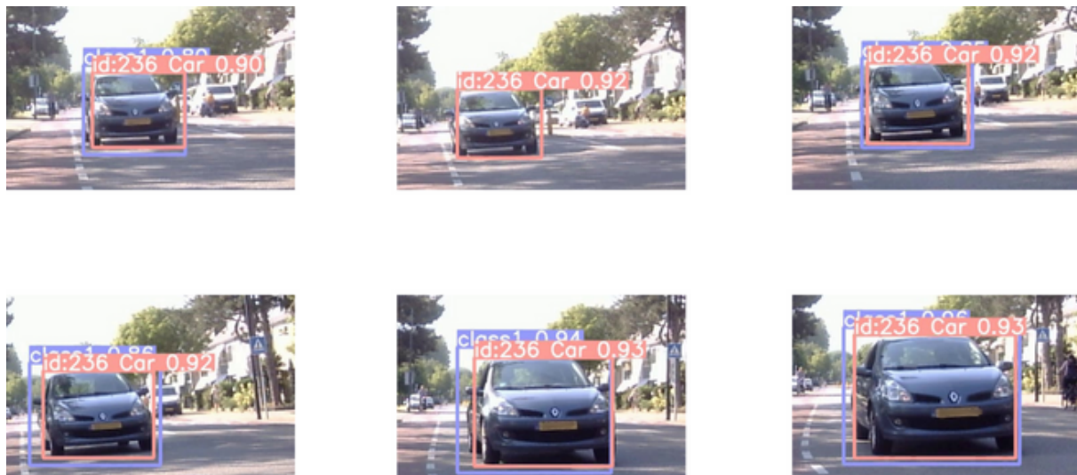
Figure 6: Frames of a video showing the tracking of YOLOv8 (bounding boxes displayed in orange, with a tracking ID) and the SAS Entity Tracking algorithm (bounding boxes displayed in blue without tracking ID).
