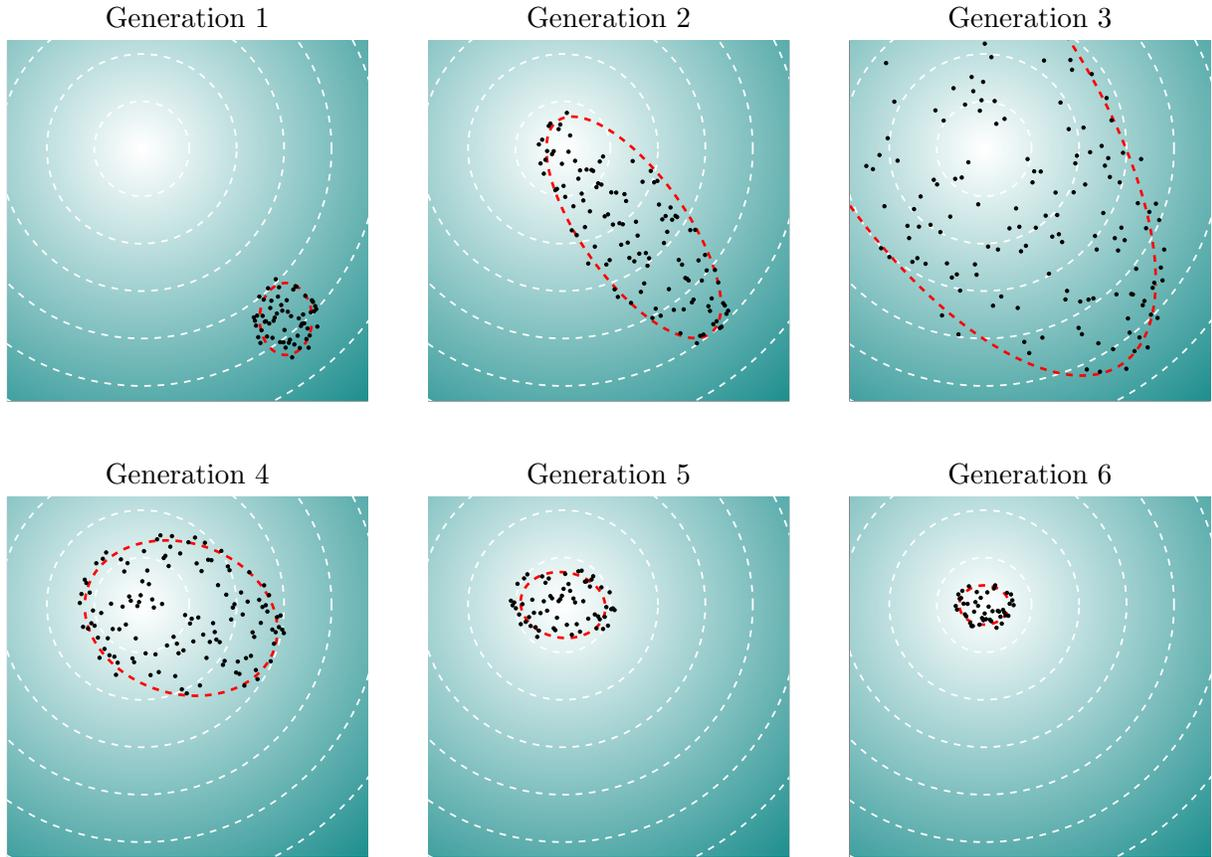
Figure 1: CMA-ES algorithm. The population is sampled from a multivariate distribution. The distribution leads the population to the global optimum.
