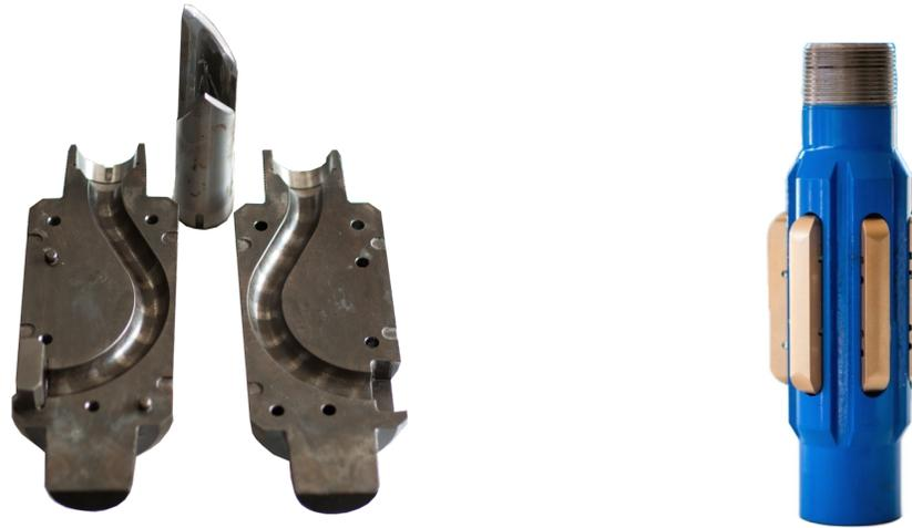
Figure 1: A cross-section and side-view of the shoe. The shoe is (in the displayed orientation) inserted into the existing well and serves as a guide to drill the hole in the existing casing at the desired location and, afterwards, for the jetting-nozzle to enter the reservoir<sup>4</sup>.
