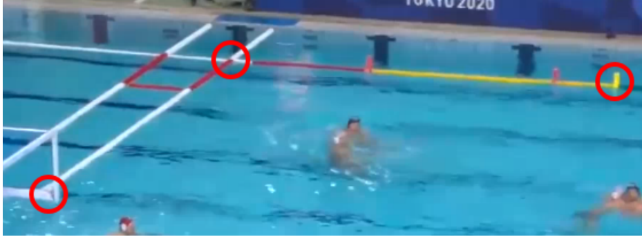
Figure 4: The three target points that can be used to apply a reverse perspective transform
