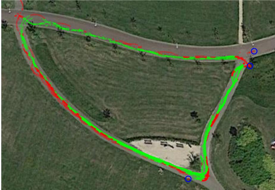
Figure 10: A visualization of the path driven by the drive model. Green squares represents recorded positions within the allowed path, red squares are outside of the recorded path. Blue circles represents points where we needed to intervene as the car drove too far of the path. A single intervention top left was outside of the bounds of the map.
