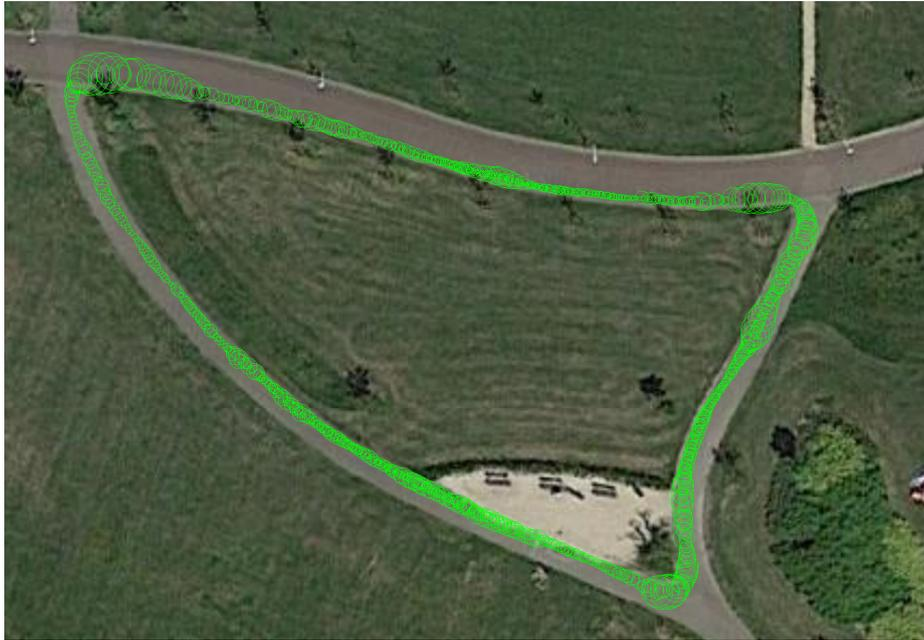
Figure 9: A visualization of the allowed path. Each circle represents a point on the curve with the radius being the allowed distance from the point. The allowed distance is determined using human driving trajectories. The allowed distance is the distance the human driven trajectories deviated from the mean path.
