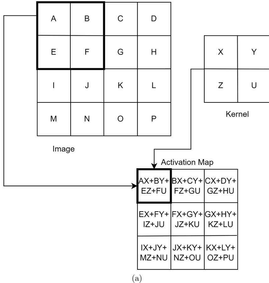
Figure 2: A visual representation of the Convolutional Layer.
