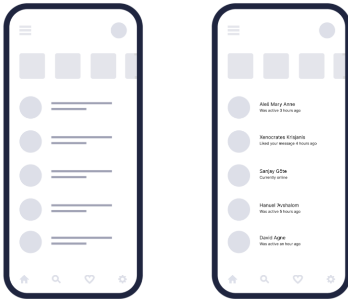
Figure 9: Mobile wireframe variants of the same social media interface. Variant A on the left has lines representing the text while variant B on the right has text included.
