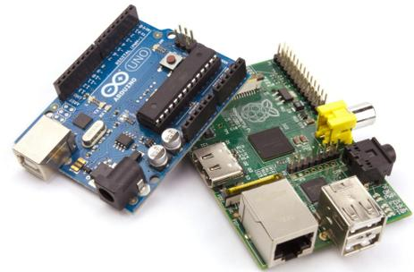
Figure 2: Arduino (left) and Raspberry Pi (right)
