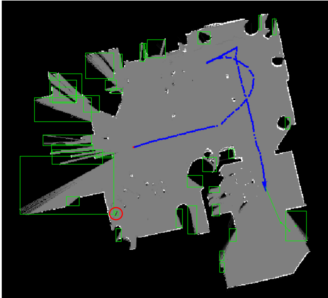
Figure 5.10: This figure shows frontiers on a partially mapped living room. The green boxes are bounding boxes denoting places of interest. The blue trail shows path taken by the robot to map the room. The green lines, show a path to a frontier. This selected frontier is chosen to be visited next by the autopilot, it is clear that an observation at the location of this frontier, yields new insight of the environment.
