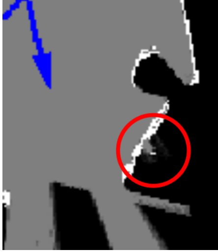
Figure 4.6: This figure shows misplaced points behind a wall. Our flood fill cleanup pass attempts to remove such points.
