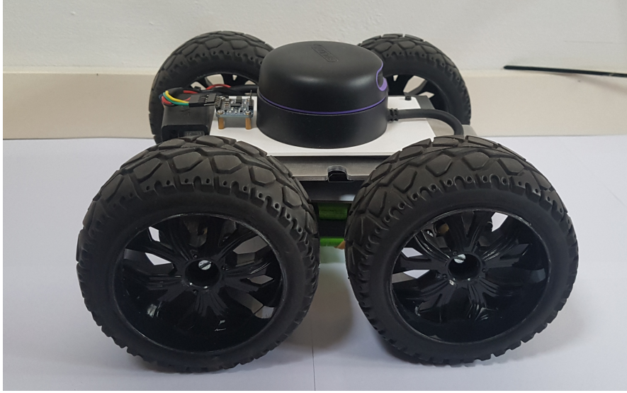
Figure 3.1: This picture shows the robot we used during our research. The LIDAR is attached on top of the robot. The IMU is placed behind the LIDAR on the small PCB.
