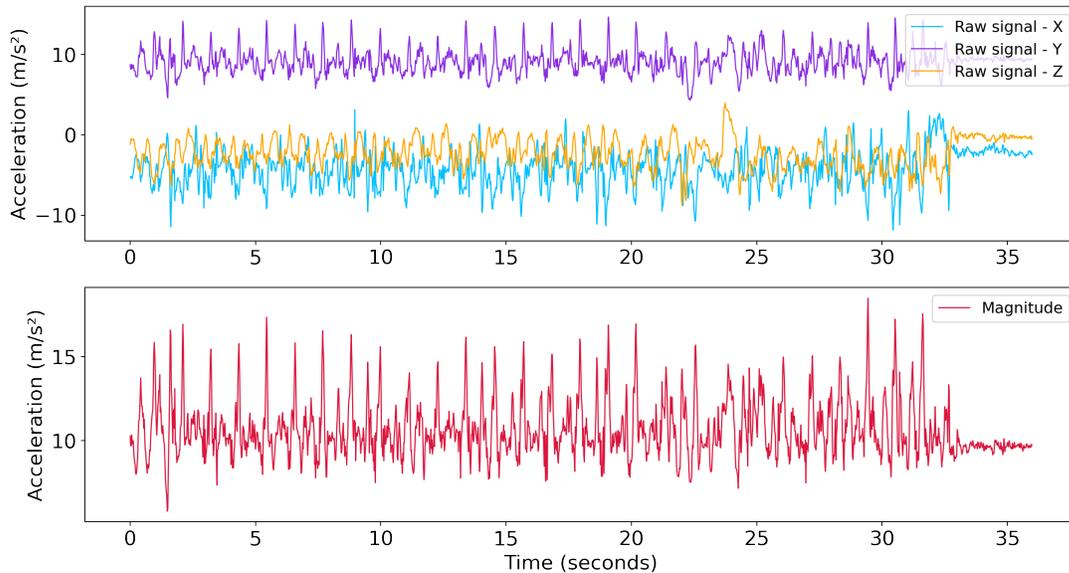
Figure 4: Raw acceleration signals from one instance of an in-clinic task. The top plot shows raw  $X - Y - Z$  signals in blue, purple, and yellow, respectively; the bottom plot (red) shows the magnitude of those signals.
