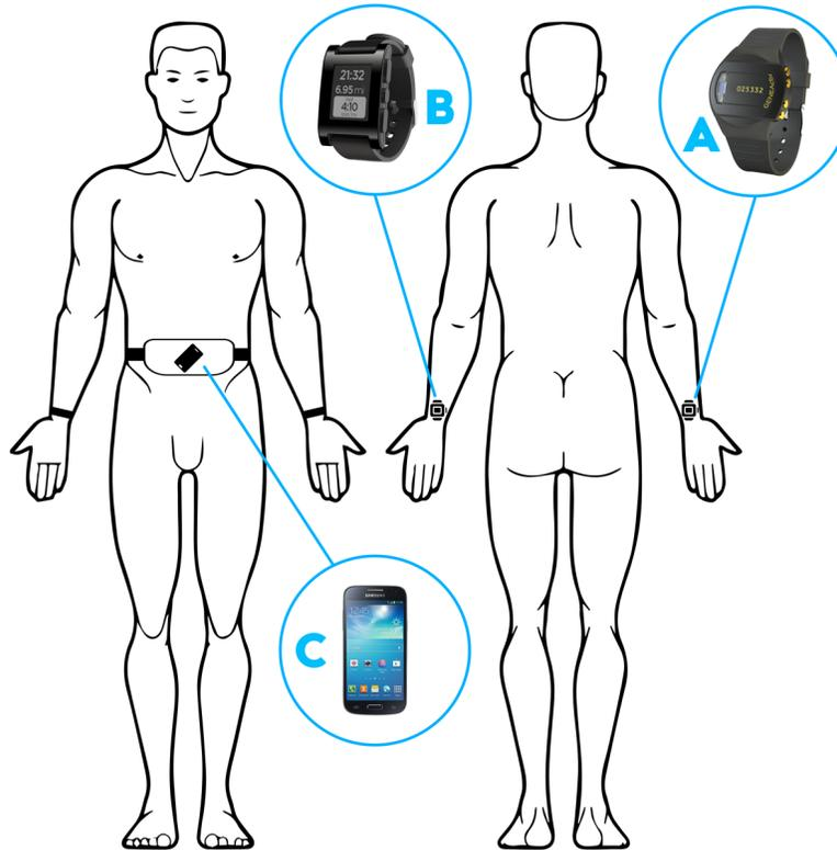
Figure 3: Sensor locations on participants. **A** - GENEActiv raw data accelerometer, **B** - Pebble Smartwatch, **C** - Samsung Galaxy Mini. **NOTE:** The sensors on left and right wrists were interchangeably used depending on the most affected side of the patient.
