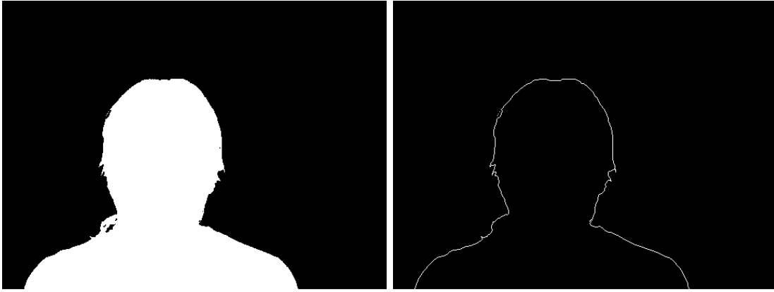
Figure 5: (left)Mask created using a threshold function on the thermal video. (right) Contours of the mask(left)
