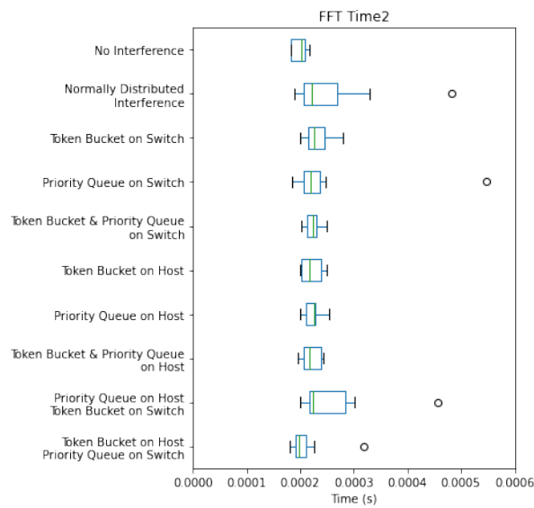
Figure 63: The results of the HPCC FFT Time2 benchmark show that the combination of the on-host token bucket and the on-switch priority queue slightly increase performance at similar consistency when compared to results utilizing other combinations of traffic shaping techniques. It seems to improve over the normally distributed interface baseline.
