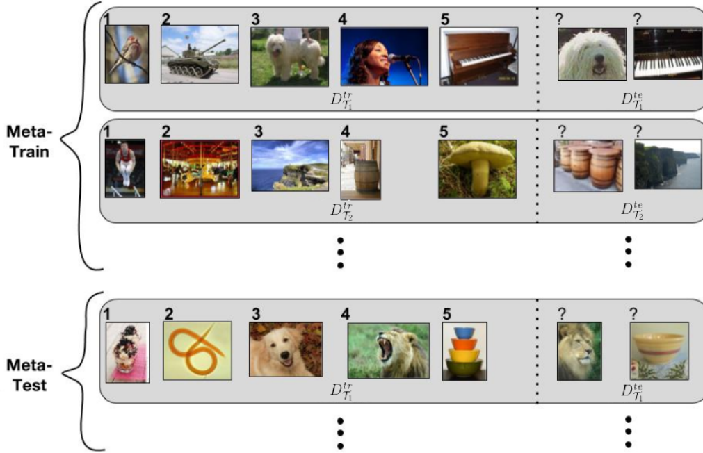
Figure 2: The N -way k -shot classification setup. Every box corresponds to a task consisting of a support set (left split) and query set (right split). There are N = 5 classes in every support set and k = 1 example per class. Note that the meta-validation stage is not displayed. Adapted from Ravi and Larochelle (2017)
