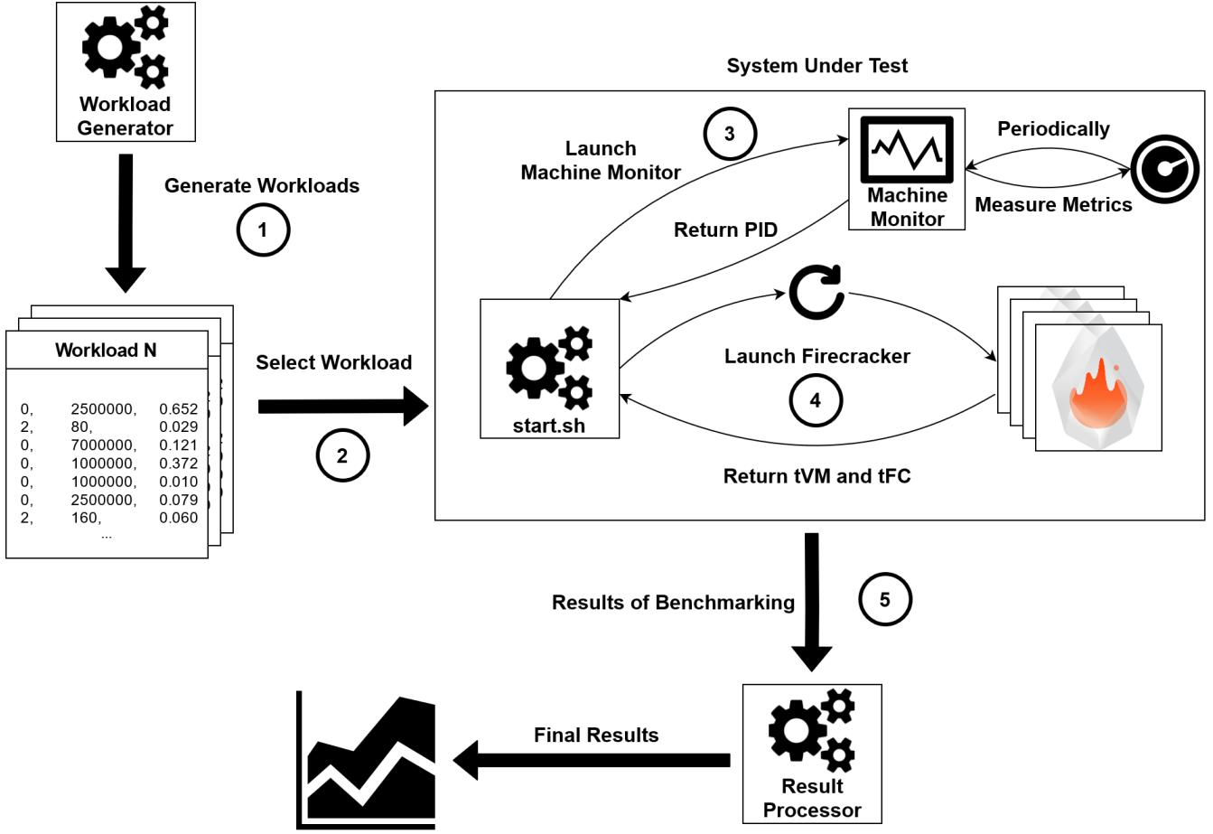
**Figure 5:** A detailed view on the working of the fc-microbenchmark.
