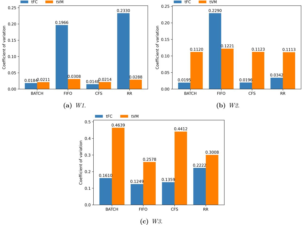
**Figure 12:** The coefficient of variation for the three workloads we analyse in this section. The vertical axis shows the value for the coefficient of variation, which is unit-less. As we measure both the run-times of the Firecracker instance and the job, there are two values per scheduler for the coefficient of variation.
