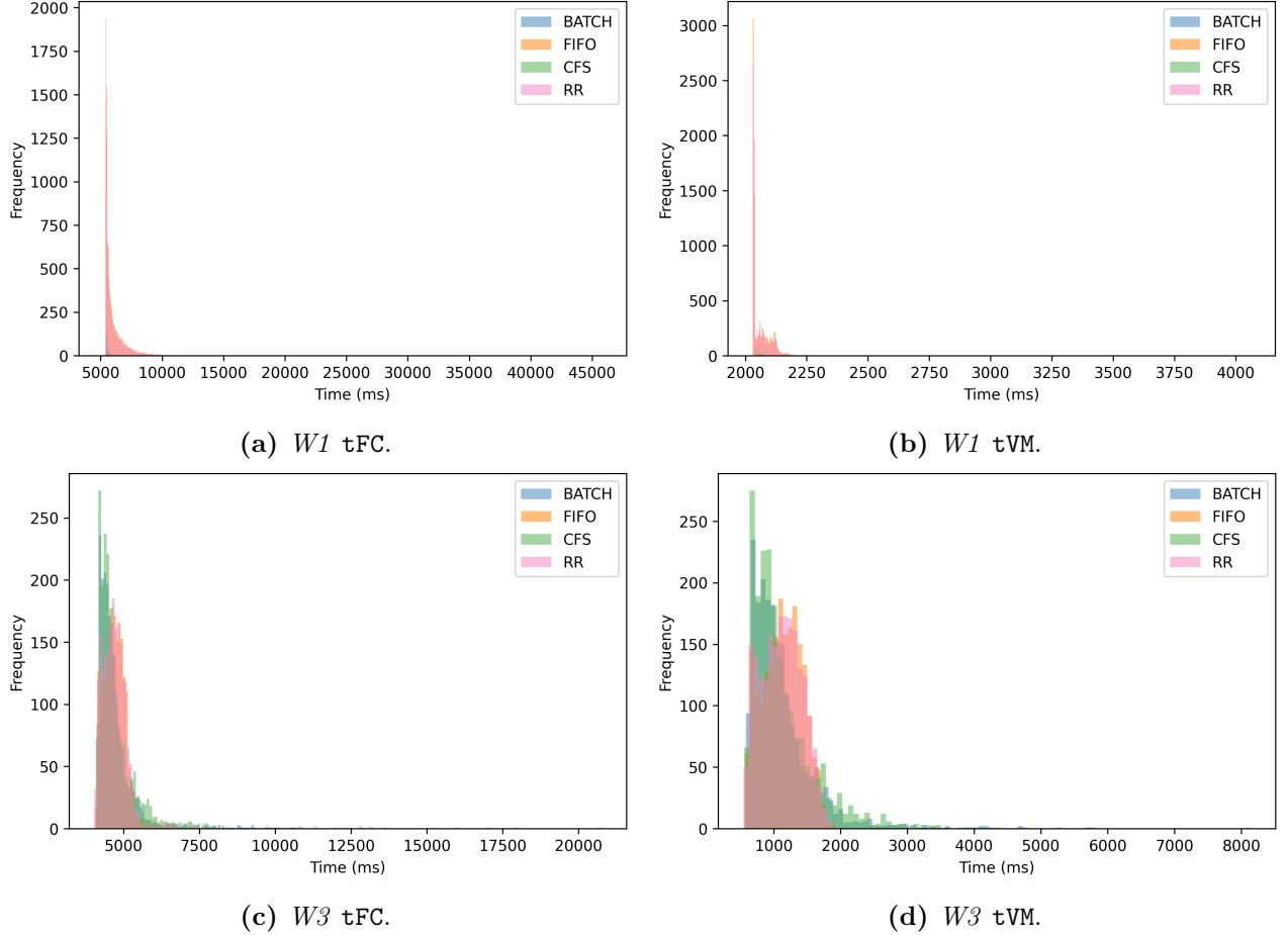
**Figure 21:** The histogram of the individual run-times of the selected program for workloads  $W1$  and  $W3$ . The bin size is determined by the Freedman-Diaconis rule [11]. The vertical axis shows the run-time in milliseconds.
