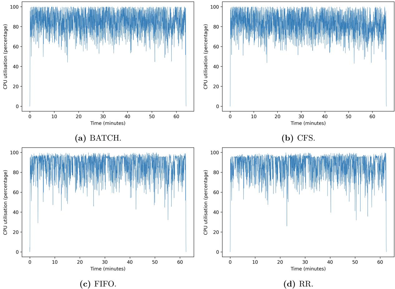
**Figure 10:** The CPU utilisation over time for all schedulers when executing workload  $W1$ . The vertical axis shows CPU utilisation as a percentage.
