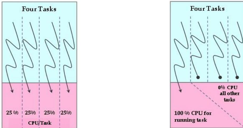
**Figure 2:** An illustration of the distribution of resources on an ideal multi-tasking single-core CPU on the left and a non-ideal CPU on the right. On such an ideal CPU, each task gets an equal slice of CPU power. Also, the tasks run truly parallel. However, a real-life CPU cannot run tasks truly parallel, as illustrated. Retrieved from: <https://www.linuxjournal.com/node/10267>.
