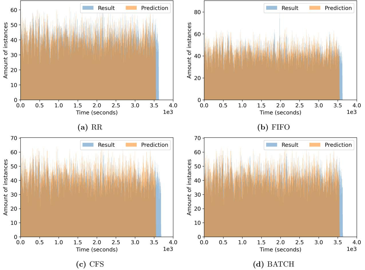
**Figure 16:** The amount of concurrent instances per unit of time of the four different schedulers for workload  $W2$ . The selected unit of time to bin concurrent events in, is 1 second. For CFS, the prediction expects more concurrency in each bin, than the results shows. For BATCH, FIFO and RR, the predicted concurrency and the actual concurrency differ less.
