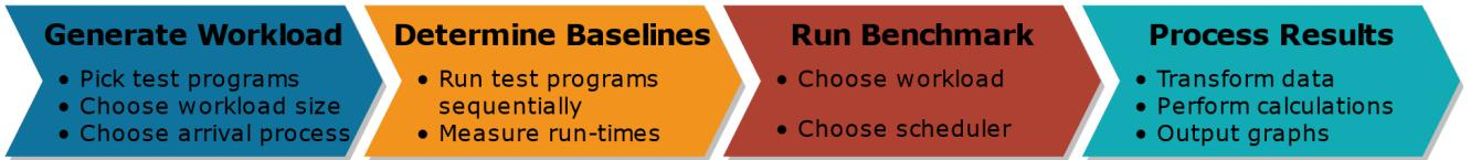
**Figure 3:** The step-by-step workflow of the benchmark for the end-user.
