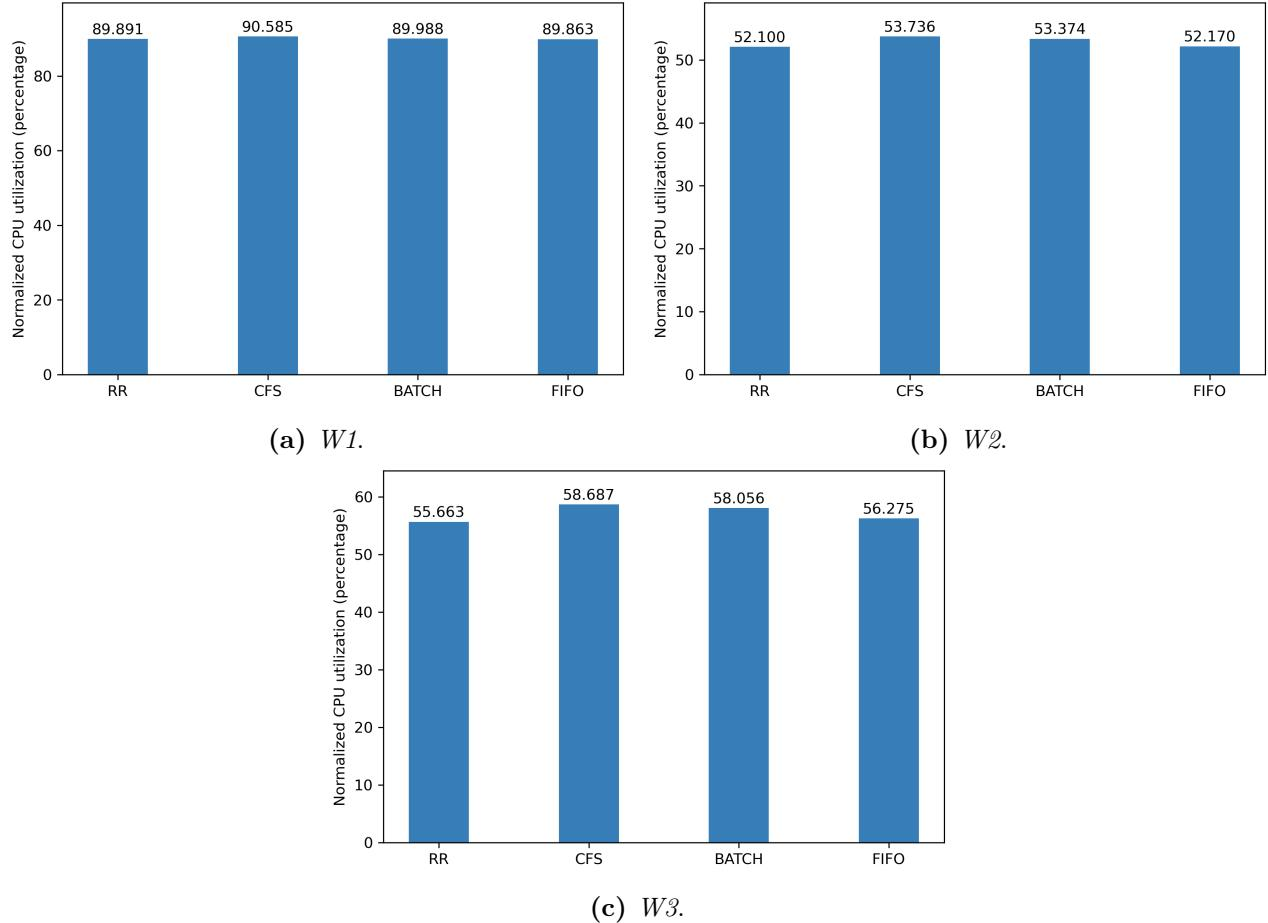
**Figure 11:** In this figure, we show the area under the curve (AUC) of the CPU utilisation of all four schedulers for the three workloads. The *maximal usage* refers to the value retrieved for a 100% CPU usage for one hour. All other AUC values are divided by this *maximal usage*, for comparison.
