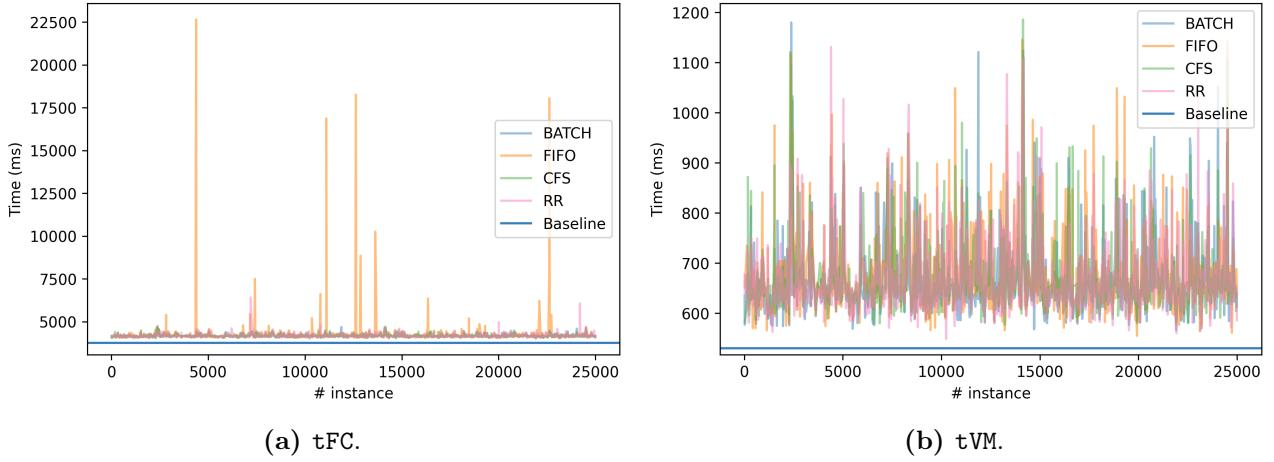
**Figure 13:** The run-time of the selected program when executing at different indices in workload  $W2$ . The horizontal axis shows the index of the program in the workload. The vertical axis shows execution-time of this program in milliseconds.
