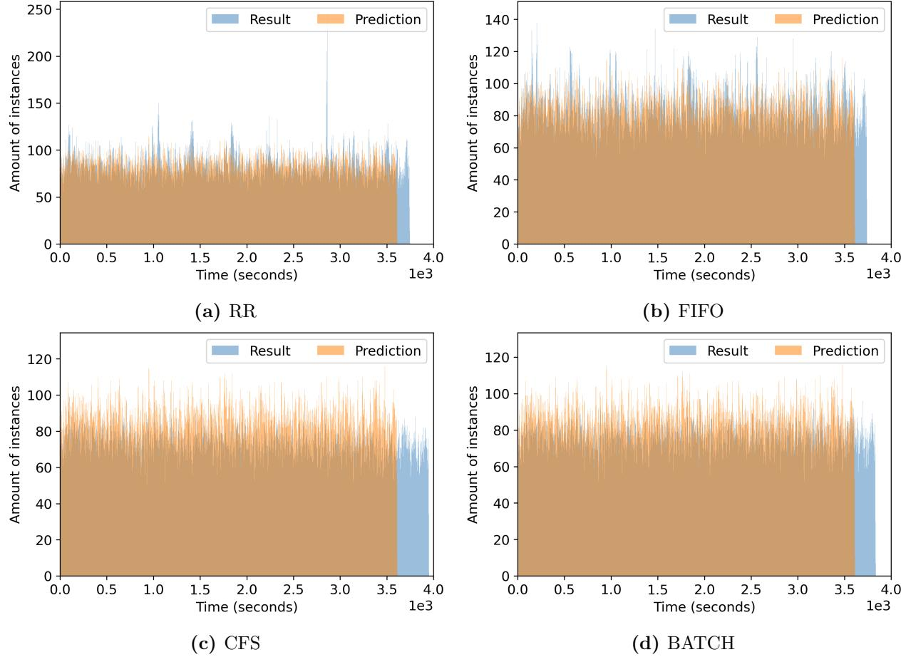
**Figure 7:** The amount of concurrent instances per unit of time of the four different schedulers for workload  $W1$ . The selected unit of time to bin concurrent events in, is 1 second. For CFS, the prediction expects more concurrency in each bin, than the results shows. For BATCH, FIFO and RR, the predicted concurrency and the actual concurrency differ less.
