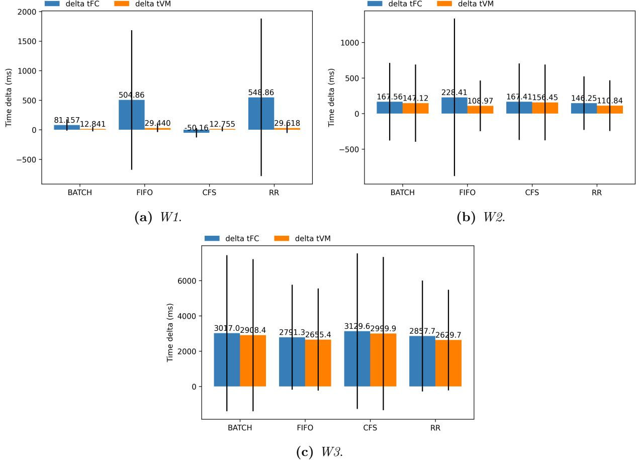
**Figure 15:** Results of the average of the calculated time-deltas for each workload and each scheduler, including the error bars.
