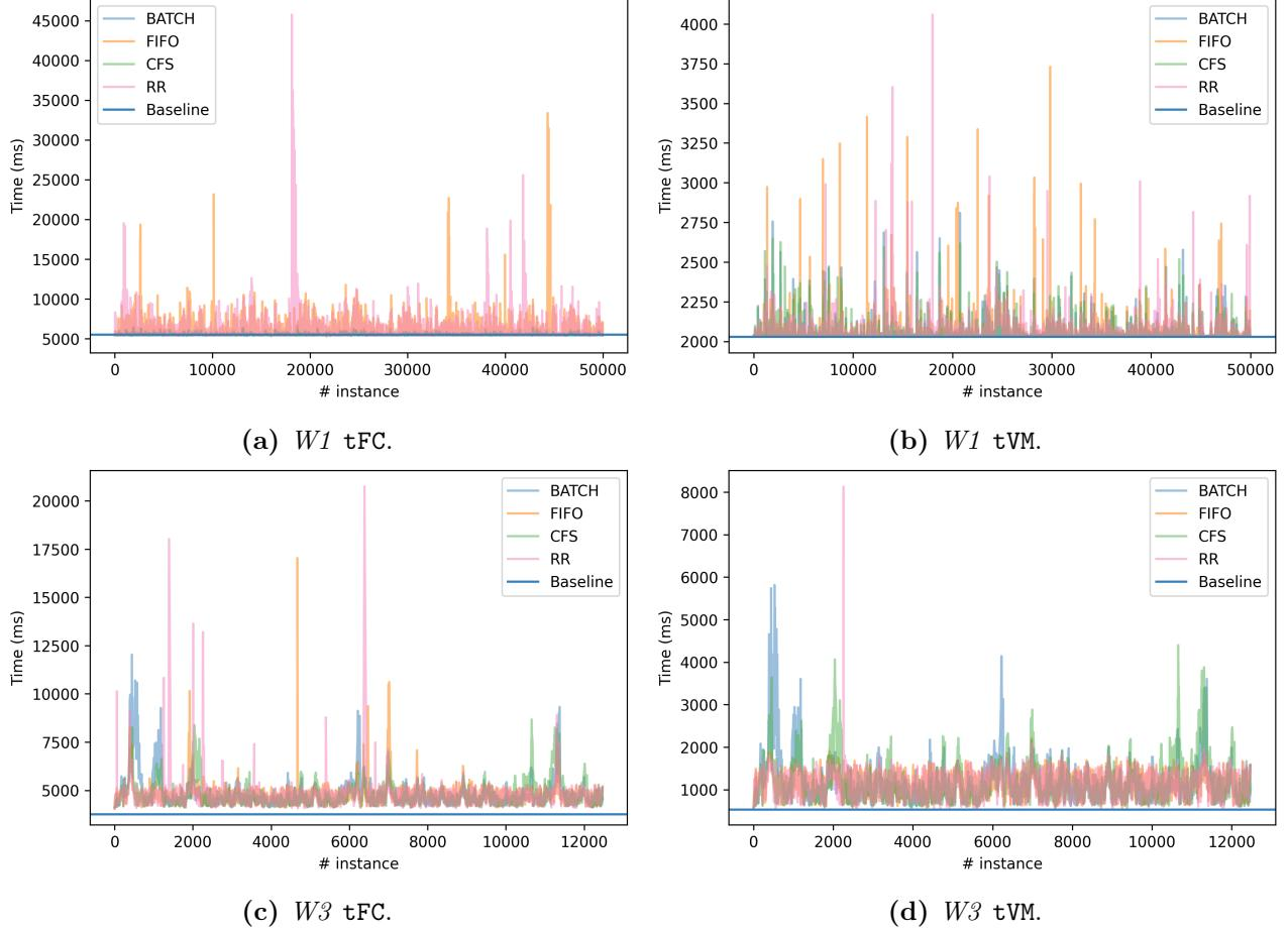
**Figure 20:** The run-time of the selected program when executing at different indices in workload  $W1$  and in workload  $W3$ . The horizontal axis shows the index of the program in the workload. The vertical axis shows execution-time of this program in milliseconds.
