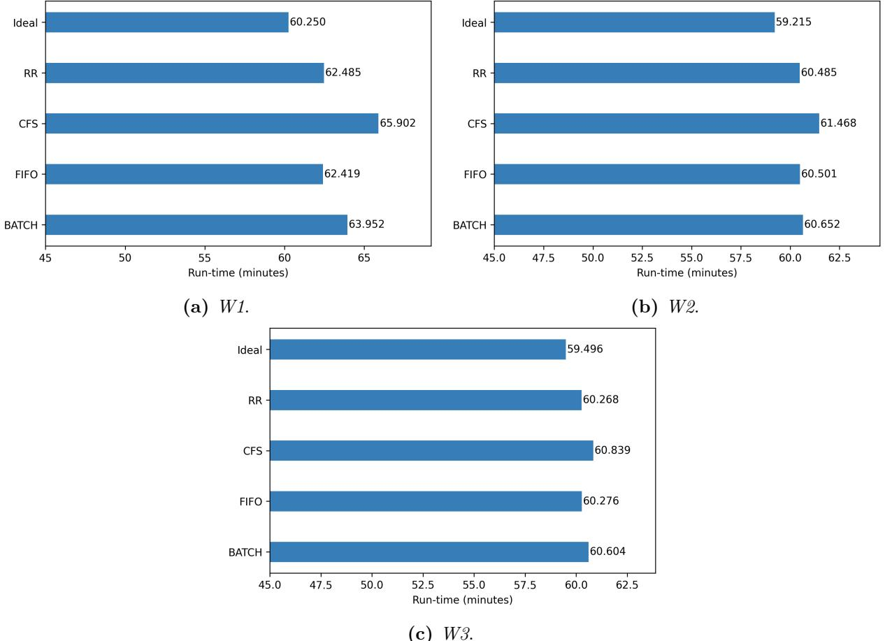
**Figure 8:** This figure shows the run-times of the workloads on the `c5n.metal` machine, in minutes. On the vertical axis, the label describes which run-time bar corresponds to which scheduler. The `ideal` is the time calculated by the prediction, as described in Section 5.3.
