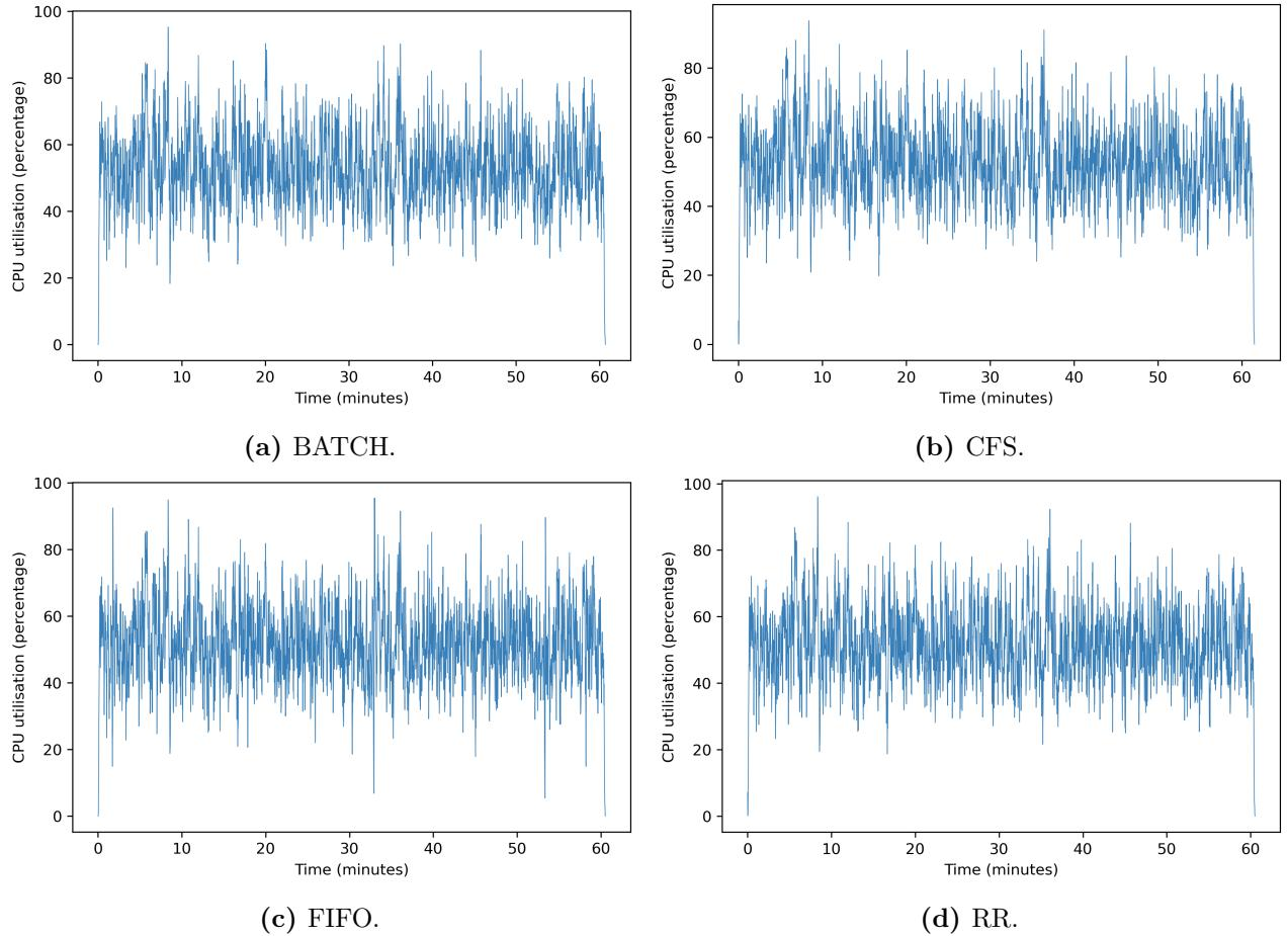
**Figure 18:** The CPU utilisation over time for all schedulers when executing workload  $W2$ . The vertical axis shows CPU utilisation as a percentage.
