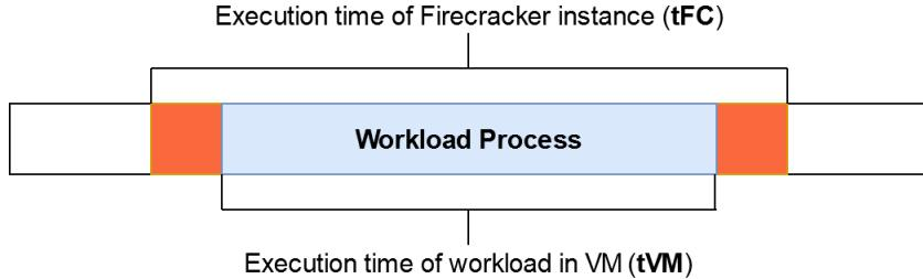
**Figure 4:** A visual representation of the  $t_{FC}$  and  $t_{VM}$  metrics.
