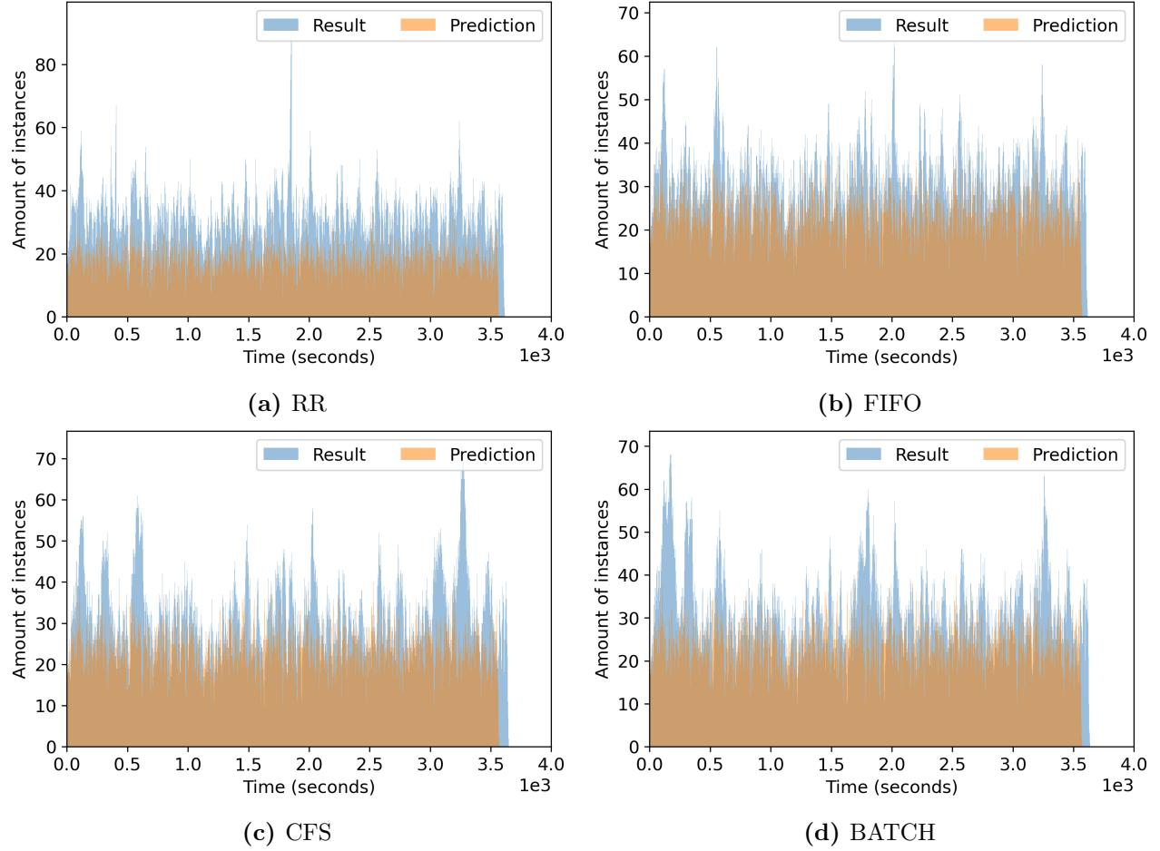
**Figure 17:** The amount of concurrent instances per unit of time of the four different schedulers for workload  $W3$ . The selected unit of time to bin concurrent events in, is 1 second. For CFS, the prediction expects more concurrency in each bin, than the results shows. For BATCH, FIFO and RR, the predicted concurrency and the actual concurrency differ less.
