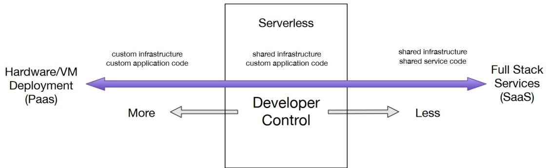
**Figure 1:** Relative control the developer has in different cloud computing paradigms. Figure taken from Baldini, *et al.* [6].
