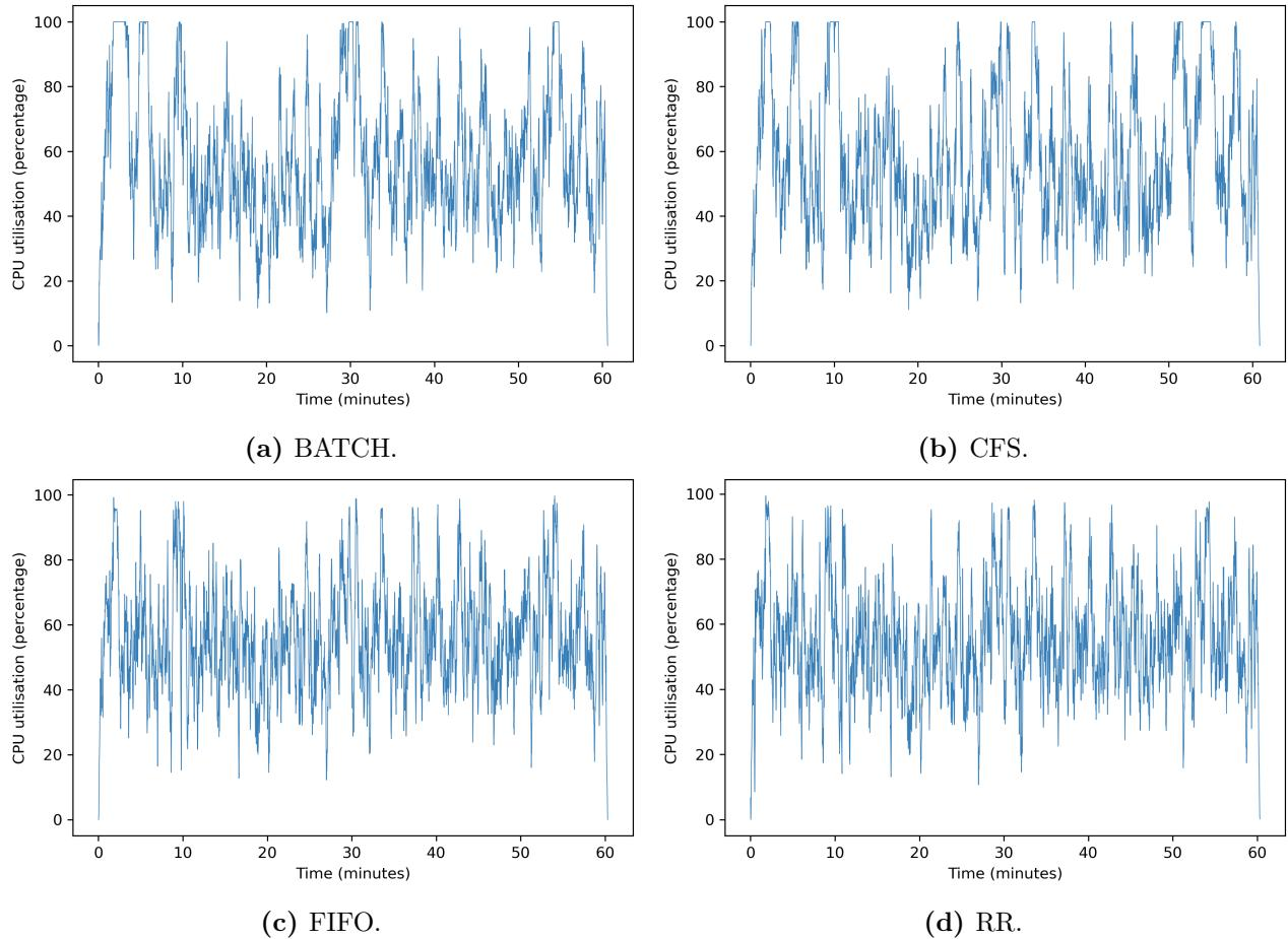
**Figure 19:** The CPU utilisation over time for all schedulers when executing workload  $W3$ . The vertical axis shows CPU utilisation as a percentage.
