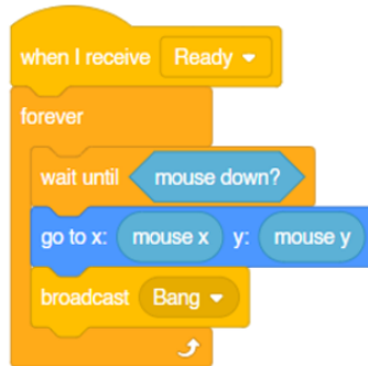
Figure 1: The code of “Fireworks display” by user ‘Dangerousgame’, which starts fireworks on a click.
