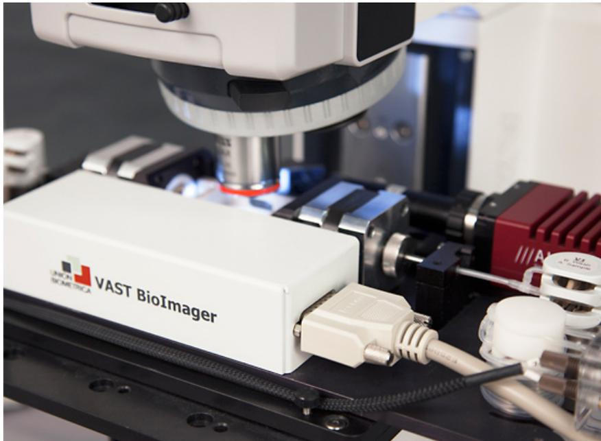
Figure 2.2: The core of the VAST BioImager, mounted on a microscope. Source: <https://www.unionbio.com/vast/>.
