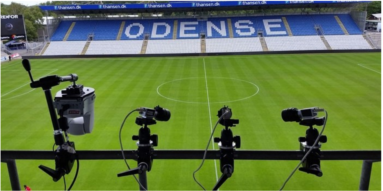
Figure 2.1: setup of the cameras to obtain position data through video analysis (adapted from https://www.stats.com/sportvu-football/ ).
