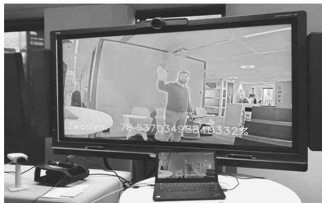
Figure 2. The AI module detects that a person is waving with an accuracy of 78.54%.
