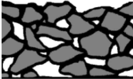
**Figure 2.1:** Illustration of the intersection of porous asphalt (ZOAB) in the Netherlands. Adapted from [50]
