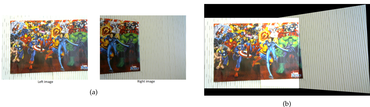
Figure 6.2: Result using RANSAC with SURF at a 22.5^\circ angle. (a) Input images; (b) Resulting panorama. The area highlighted in green is the sweet spot.
