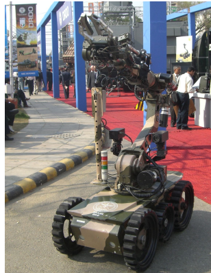
Figure 1.2: Daksh is an electrically powered Remotely Operated Vehicle (ROV) designed and developed by the Indian state-owned Defence Research and Development Organisation (DRDO) at the Research and Development Establishment (Engineers), Pune, India [49].
