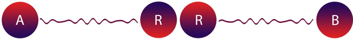
(a) The qubits in the network nodes of Alice (A) and Bob (B) first generate entanglement with the repeater node (containing two qubits) in the middle.
